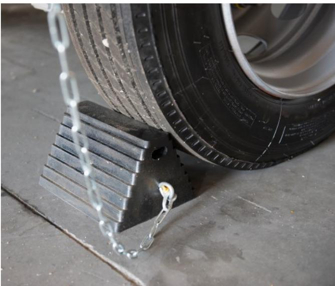
4. When stationary place the chock firmly under the wheel and return to the chock hook when towing.
