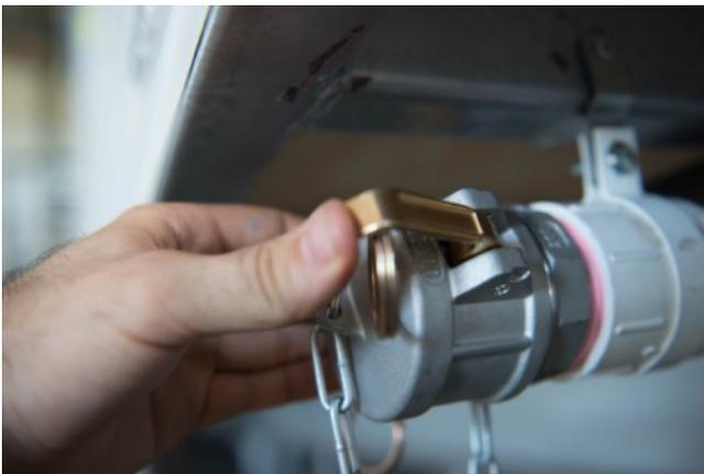
2. Access the inlet cap by pushing back each latch and attach your hose to the 50mm cam lock fitting.
