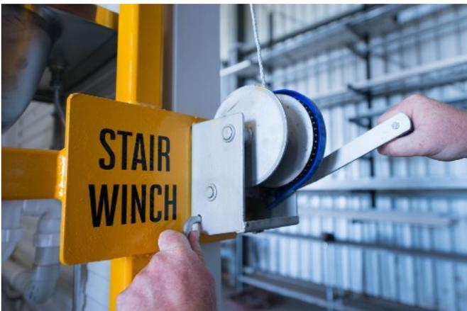
2. Ensure that the ratchet latch is engaged and locked in position and that the winch cable is taught through the pulley and winch.
