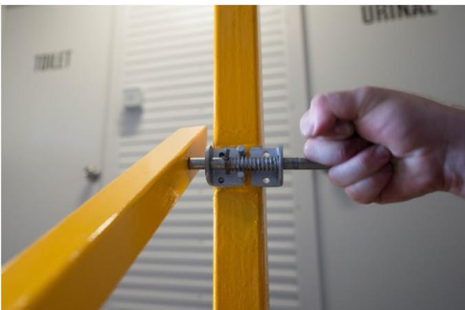
7. Lock the stairs in place with the locking mechanism located on each handrail. To erect the the stairs reverse this process.
