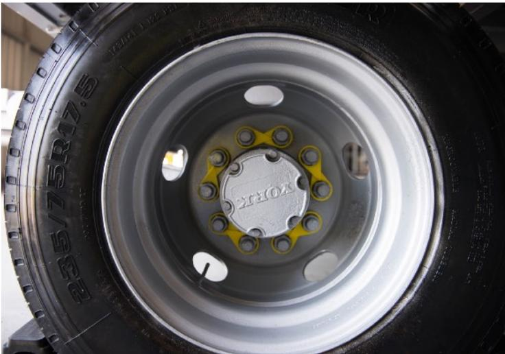
Check the wheel nuts of each wheel are aligned before towing.
