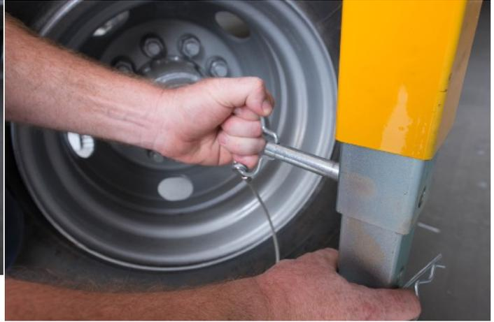
4. Lower the jack extension leg to a suitable level (The ground or stable surface) and then re-insert the pin to lock in place with the small pin.
