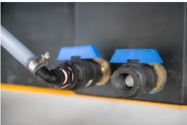
2. To close the drain rotate the valve 90 degrees so its horizontal to the water tank. Note this valve can also be used to fill up the water tank with the correct fitting.
