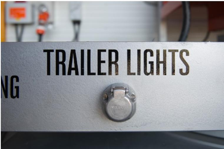
Before towing ensure that the trailer lights are connected.
