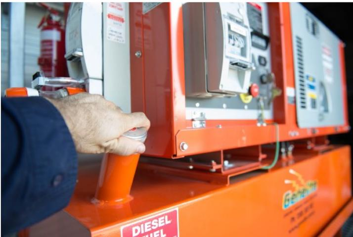
2. To access the tank unscrew the cap.
