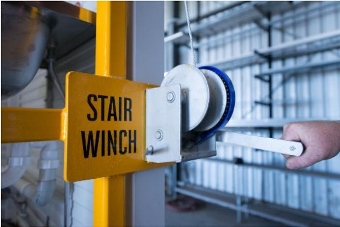
4. Release the ratchet latch and slowly lower the stairs towards position on the ground.
