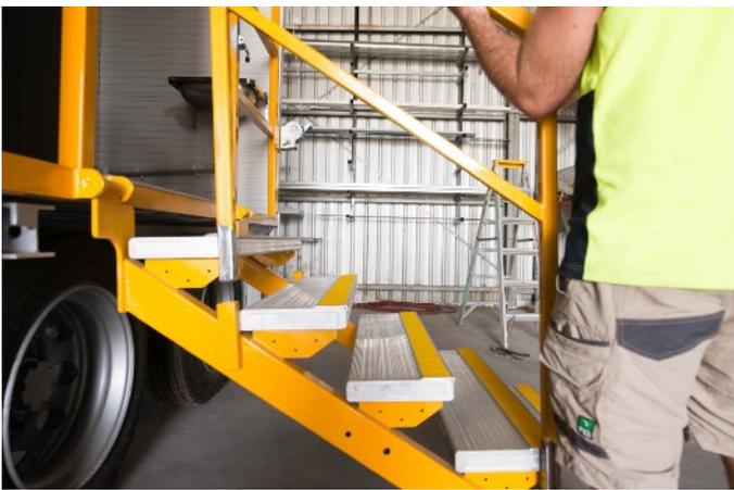
8. Line up the corresponding handrail with the handrail stabiliser points, there are 2 located on each side of the stairs and insert them.
