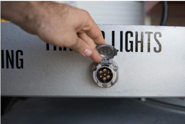
2. Flick the connector cover back and insert the trailer connector.
