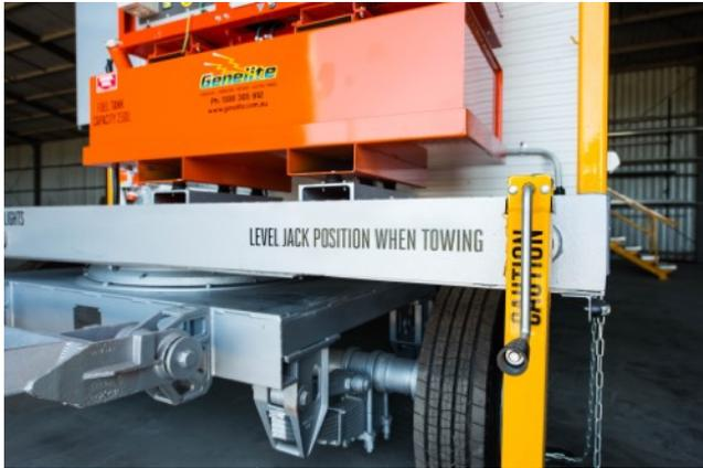
1. Locate the 4 jacks on each corner of the mobile crib room (Note there is also a levelling jack on the A-frame boom at the front).
