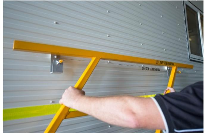
7. Locate the left and right step hand rails and unscrew them from the holster.
