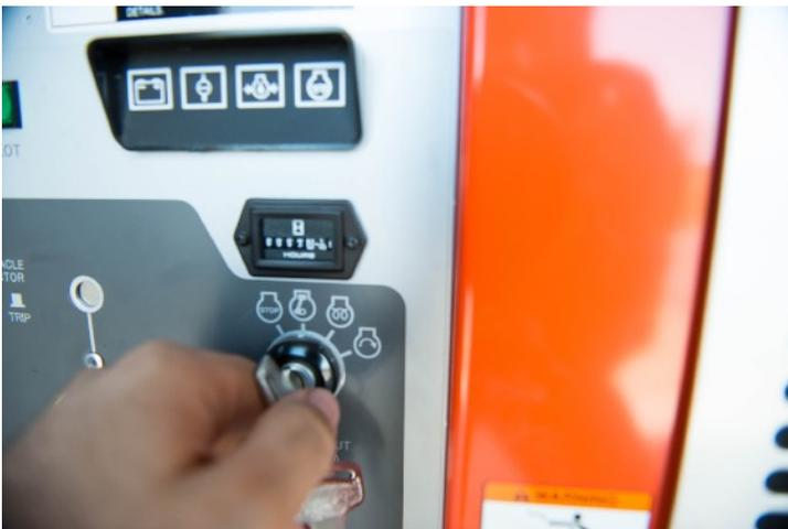
5. Turn the key right 2 stages (the glow symbol) leave this here until the glow light in the above indicator display turns off. This allows the engine time to warm up.
