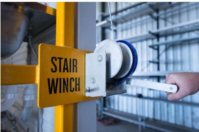
6. Rotate the winch handle to bring the hook up to the pulley and then lock the ratchet for the final time.
