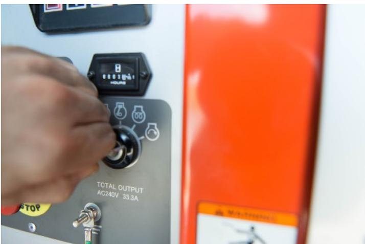
6. Once the light disappears turn the key fully to the right to start the engine. To turn it off turn the key to the left.
