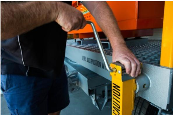
5. Rotate the jack handle to raise the jack to a suitable height.
