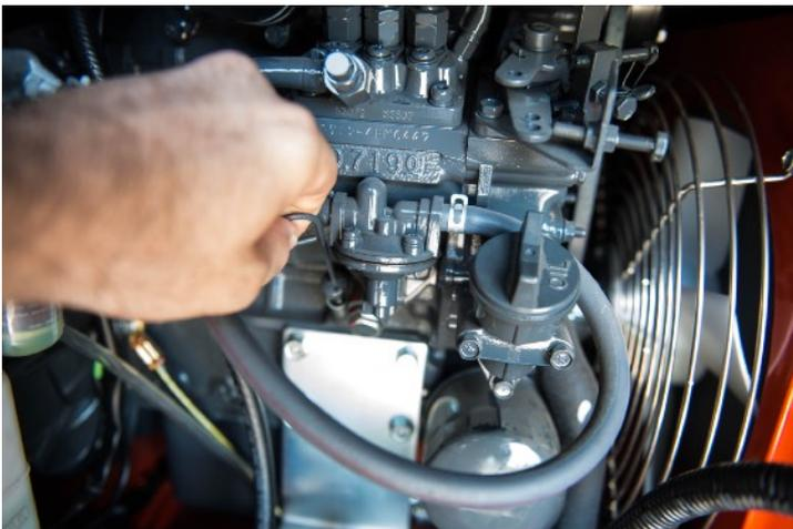
3. Locate the oil dip stick, pull it out. and check the level as per the instructions in the user manual index.
