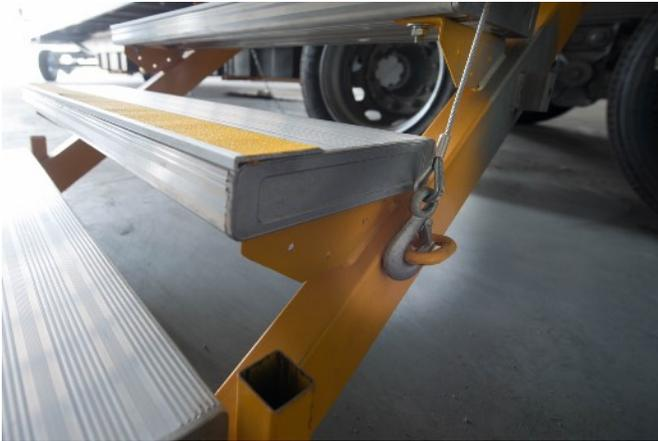
1. Ensure that the hook is locked to the lifting loop on the lower right section of the stairs.
