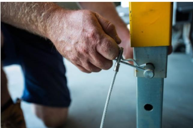
3. Remove the small jack extension leg pin so you can pull the larger leg pin out.
