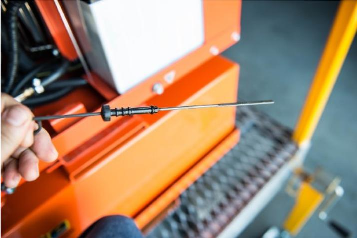
4. Check the level on the dip stick as per the directions in the user manual index.
